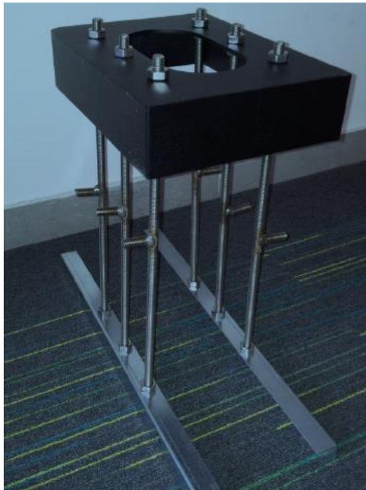
Figure 4: Assembled underground anchoring element
