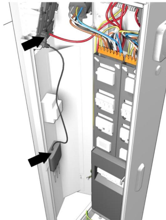
Figure 25: Connecting the UTP cables
