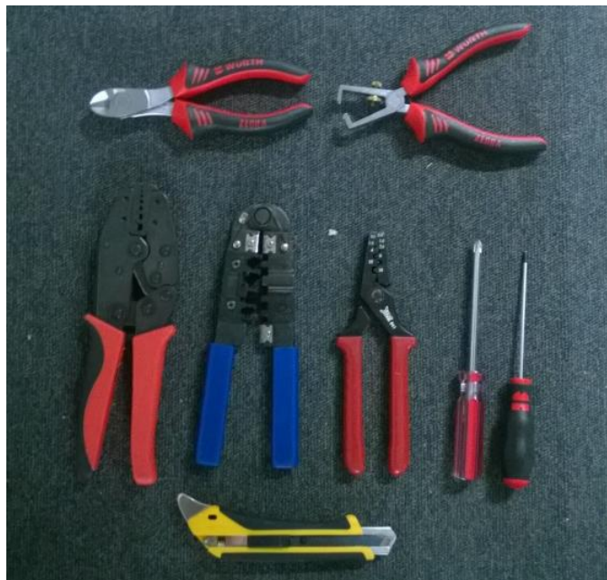
Figure 42: Equipment used for the installation of charging station
