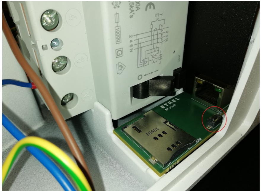
Figure 7: Reset button inside the maintenance opening
